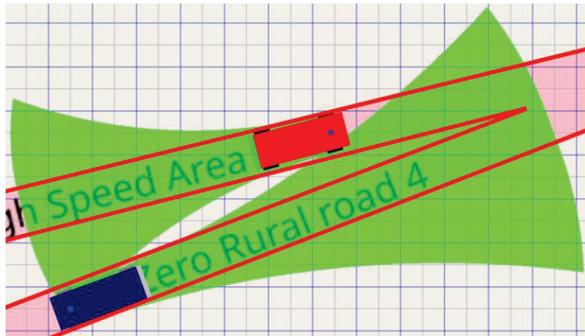
Figure 40 Two vehicles meeting each other as in the previous figure, but safety zone is only applied to their respective lanes
