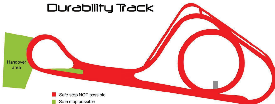
Figure 50 Safe stop concept at Durability Track, Hällered Proving ground
