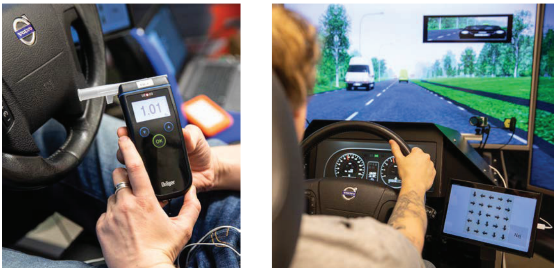
Figure 6. The breath alcohol measurement equipment (left) and the NDRT performed while driving in the simulator. Photos: Katja Kircher.
