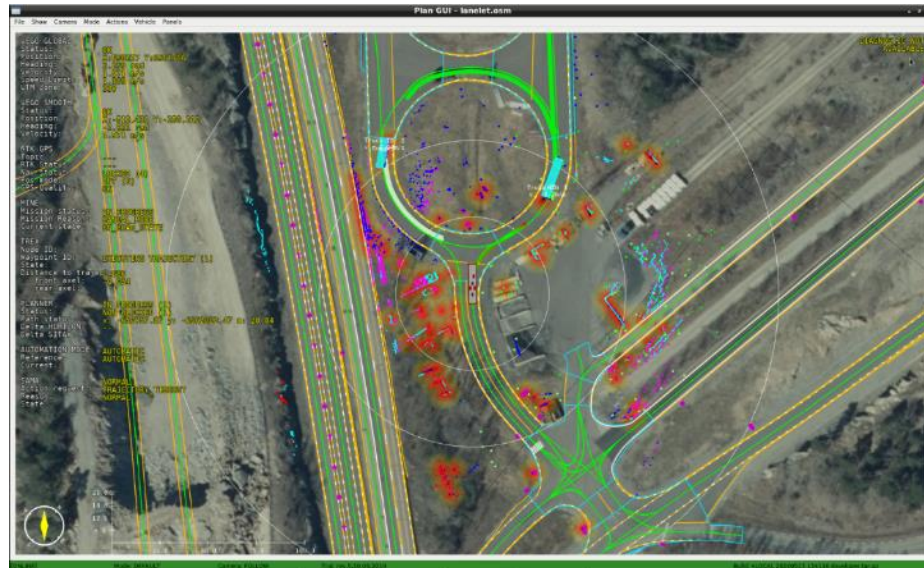
Figure 9 – PlanGui. The onboard HMI system
