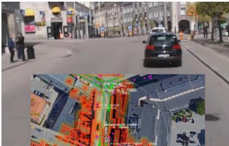
Figure 32 – Example of static obstacle detection from 3D lidars after removal of the ground plane in central Södertälje, Black areas surrounded by red are areas detected as static obstacles by the vehicle.
