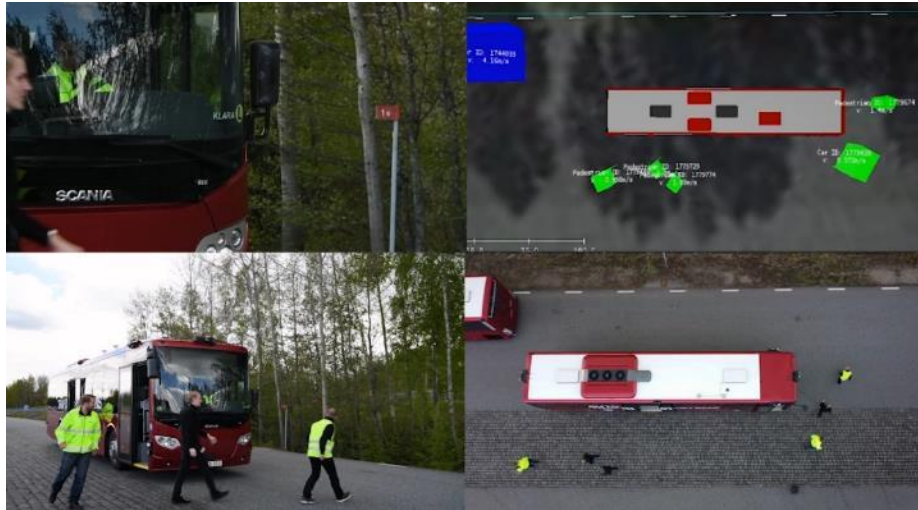
Figure 27 – Multiple high level pedestrian objects around an iQPilot vehicle and the real world situation
