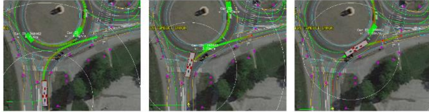
Figure 43 - An example of the prediction system being interfaced with the Scania system. In this case the predicted gap between the agents is too narrow, and the planner produces a yielding manoeuvre.
