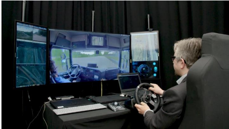
Figure 7 – Remote Drive Demonstration. The demonstration comprised a control station, forwards view in the vehicle, strategic map information, external view of the vehicle and mirroring of on-board HMI
