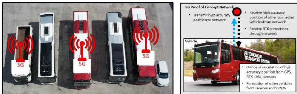
Figure 61 – 3 vehicles were connected to the 5G POC network for the final iQPilot demo. These vehicles continuously provided other vehicles connected in the network with high accuracy position information
