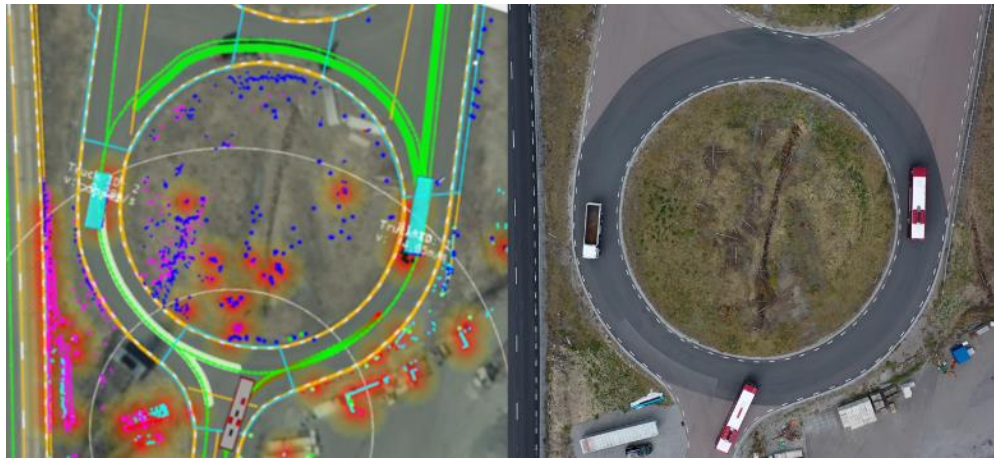
Figure 39 – Example of predicted motion of other agents in the environment based on road layout
