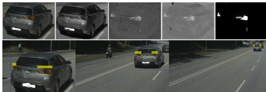
Figure 35 – Example of processing a ROI that has been classified as a car to detect and track the lights as a sub-ROI
