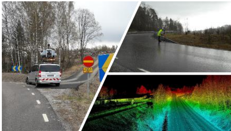
Figure 14 – Lidar (Trimble MX8) and camera data collection vehicle (left), surveying of reference points (top right) and point cloud representation of the environment (bottom right)
