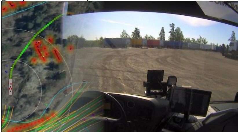
Figure 47 – Open area planner planning through an open area with obstacles on the left hand side. Real situation in forwards view camera on the right.
