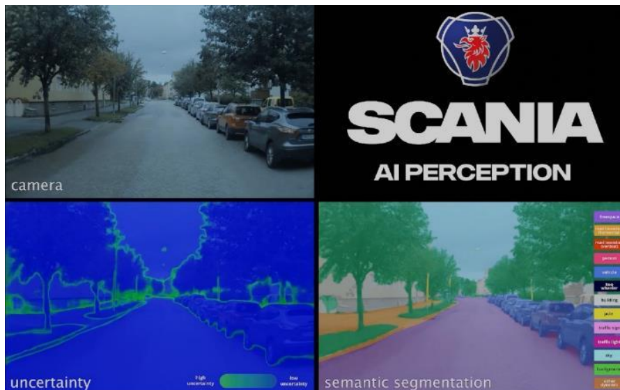
Figure 37 – Sample image segmentation and uncertainty on one of the iQPilot vehicles during a drive in Södertälje. This focus area continues with the iQDeep project
