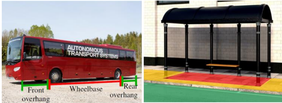
Figure 48 – Regions of vehicle characterised to segments according to wheelbase and areas with overhangs. The environment is also segmented into driveable areas according to the road layout (green), sweepable area (yellow) and obstacles (red).
