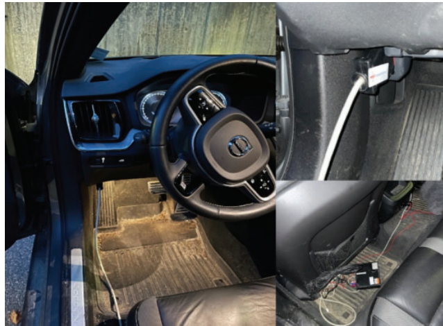
Figure 4 PPDS data collection system
