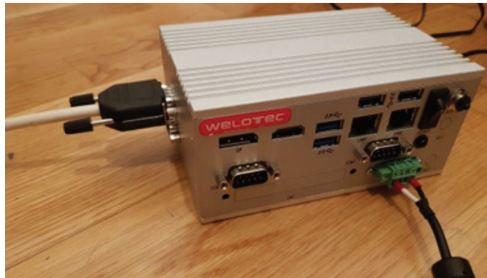
Figure 2 Picture of one Welotec Gateway with one Serial CAN connector.
