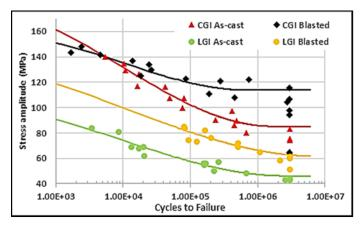
Figure 5. S-N curves for Scania CGI and LGI, in as cast and as blasted conditions. Stress ratio R ratio=  $\sim 0.15$ , runouts: over  $3 \times 10^6$  cycles.
