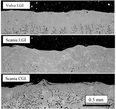
Figure 2. Cross-section of blast cleaned LGI and CGI showing casting skins.
