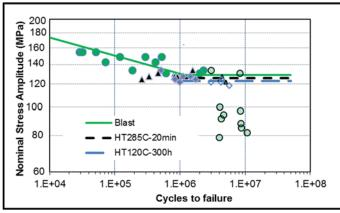
Figure 6 The effect of heat treatments on Volvo blasted LGI. R ratio=0.1, runouts: over  $3x10^6$  cycles.
