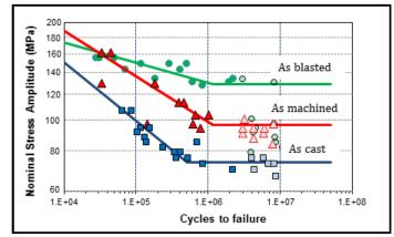
Figure 4. S-N curves for Volvo LGI. Stress ratio R ratio =0.1, runouts: over  $3x10^6$  cycles.
