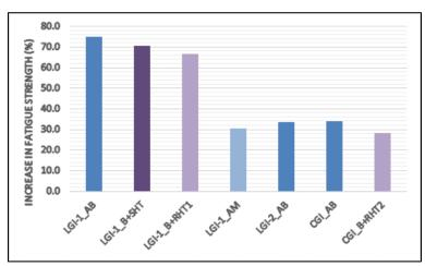
Figure 1. Improvement in fatigue limit after the different treatments. AB: as blasted, AM: as machined, B+SHT: blasting + annealing 20 min at 285 °C, RHT1: blasting + annealing 300 h at 120 °C, RHT2: blasting + annealing 300 h at 220 °C.
