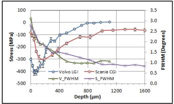
Figure 3. Residual stress and FWHM profiles in blasted LGI and CGI. XEC= $5.81 \times 10^{-6}$  MPa<sup>-1</sup>
