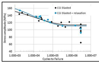
Figure 7 The effect of stress relaxation annealing (300 h at 220 °C) on Scania blasted CGI. R ratio=~0.15, Runouts: over 3x10<sup>6</sup> cycles.
