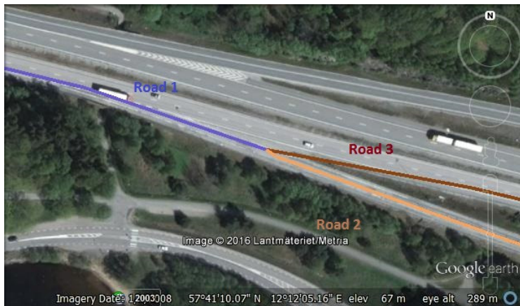
Figure 11: Road section topology and lane geometry enable improved target selection for longitudinal and lateral control
