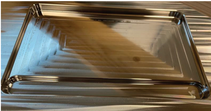
Figure 2. Tool with milled engraving
